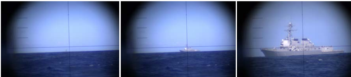
Figure 1: A tactically useful ATR algorithm will be able to classify targets by extracting key features while much of the hull remains below the horizon.
