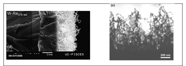
Figure 1: Formation of fuzz on tungsten surfaces exposed to an He-containing plasma. Left: exposure at 1120K, He energy=40eV [1]; right: exposure at 1400K, He energy=50eV [2].
